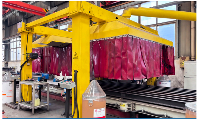
Bridge deck welding machine
