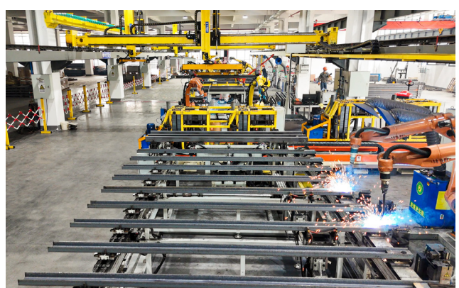
Chord welding robot production line
