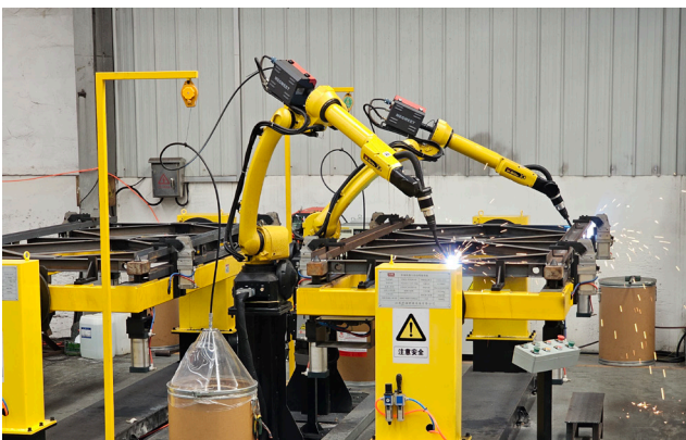
Bailey panel automatic welding machine
