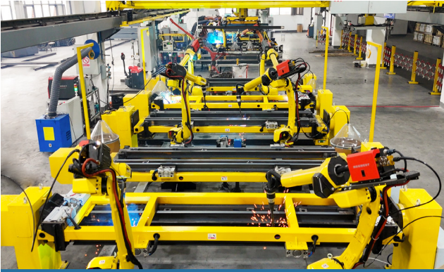
Chord automatic welding production line
